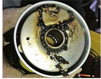
A filter clogged up with nasty diesel sludge
