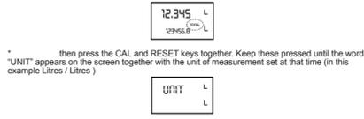
then press the CAL and RESET keys together. Keep these pressed until the word "UNIT" appears on the screen together with the unit of measurement set at that time (in this example Litres / Litres).
